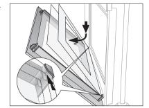
2. Take hold of the door trim (B) at each side, position it on the inside edge of the door and plug the door trim (B) into the upper edge of the door.
